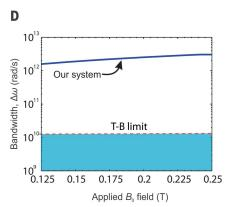
delay and storage times would be (7-15)  $\Delta t_{\rm max} \sim (\Delta \omega)^{-1}$  or less, i.e.,  $\Delta t_{\rm max} \sim 5$  ps =  $10T_{\rm p}$ . Thus, our nonreciprocal device is above the conventional delay time–bandwidth limit of state-of-the-art slow-light systems by more than a factor of 40.
