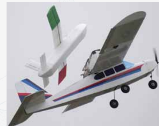
An early flight test of an ASTRA rapid prototyped glider, launched from the top of a radio-controlled 'mothership'.
